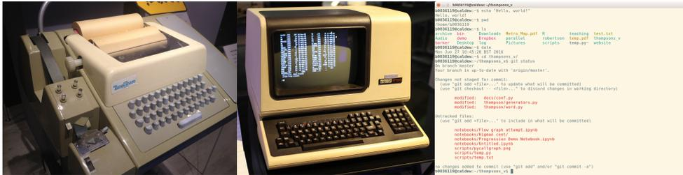
Figure 17: Left: A Teletype Model 33 ASR teleprinter, manufactured from 1965 to 1976. Centre: A DEC VT100, introduced in 1978. Right: A terminal emulator GNOME-TERMINAL. This is what ‘terminal’ typically refers to nowadays.
