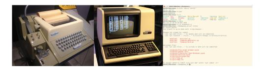
Figure 17: Left: A Teletype Model 33 ASR teleprinter, manufactured from 1965 to 1976. Centre: A DEC VT100, introduced in 1978. Right: A terminal emulator GNOME-TERMINAL. This is what 'terminal' typically refers to nowadays. Image: https://commons.wikimedia.org/wiki/File:ASR-33\_at\_CHM.agr.jpg Image: https://commons.wikimedia.org/wiki/File:DEC\_VT100\_terminal.jpg
